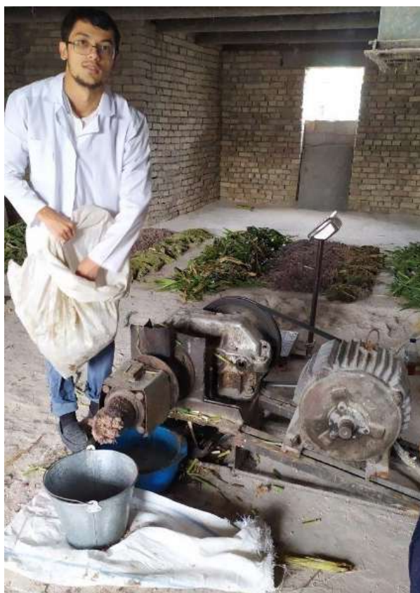
Figure 2. Obtaining juice by cutting to certain sizes and passing through a screw device
